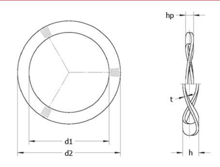
d1 = 78.30 d2 = 88.20 F (N) at hp = 300.0 For bearing = 6011, 6210, 6308, 6406, 16011 h = 3.7hp = 1.60 t = 0.50 Waves = 6 Weight (kg) / 100 pcs = 0.517
